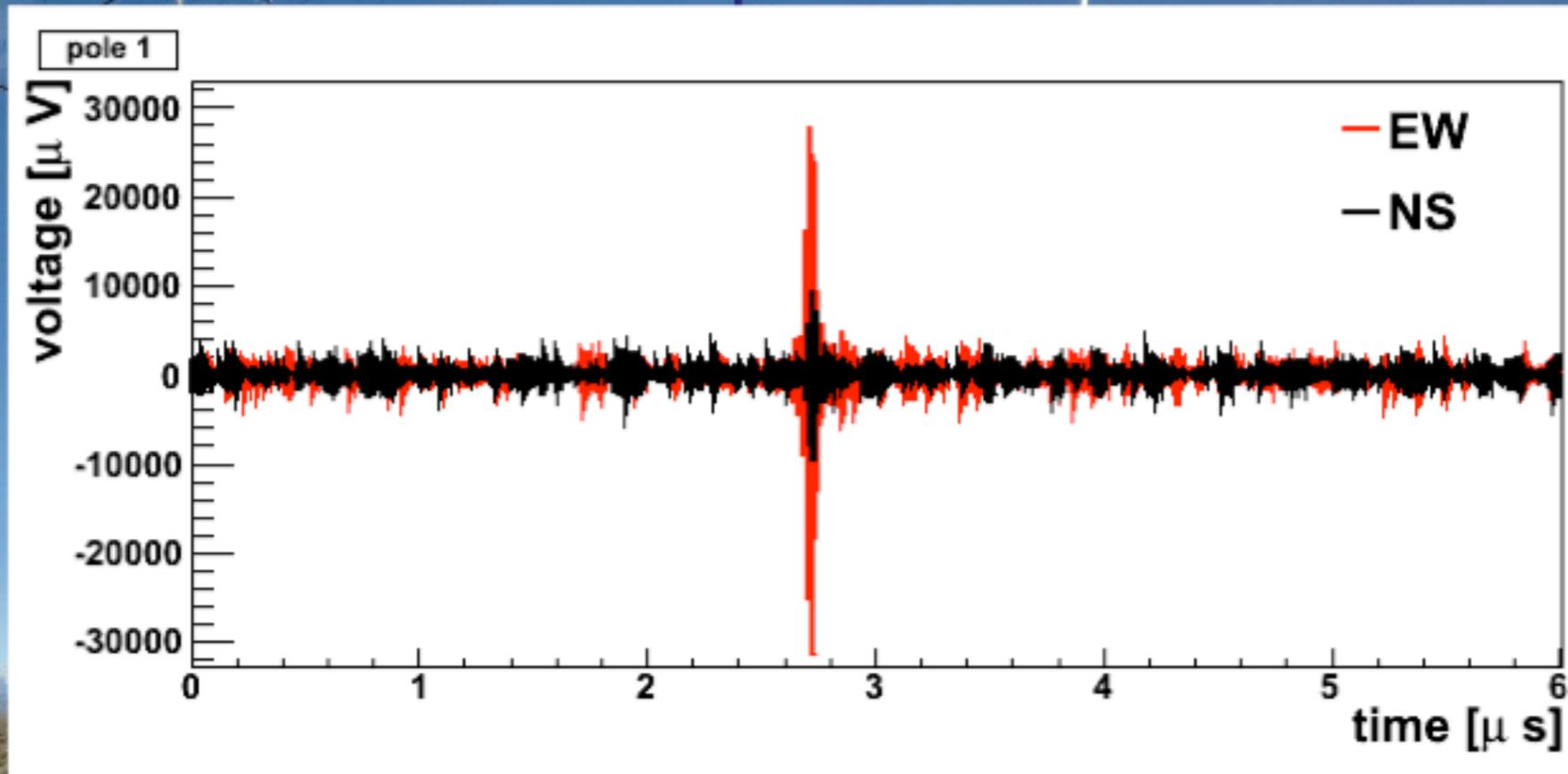
Radio signal measured in coincidence with SD
